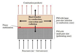
Fig. 1.Schematic diagram of two layer porous burner. media is desirable. A brief account of some basic parameters is
