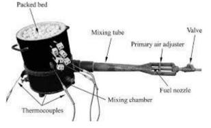
Fig. 5.SPMB developed by Yoksenakul and Jugjai (2011).
