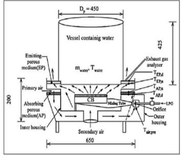
**Fig. 2.**PRRB Burner proposed by Jugjai and Sanitjai (1996). Part of thermal radiation is redirected towards the absorbing porous medium through emitting porous medium, which then preheats the primary air that flows inside the air jacket. The porous media that are used in this study are made of several layers of stainless steel wires with 40 meshes per inch.
