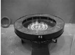
**Fig. 4.**PRRB developed by Jugjai and Rungsimuntuchart (2002). T Fend et al. (2003) paper will report on methodology and results of thermal conductivity, convective heat transfer coefficient and efficiency measurement of these monolithic materials. It will also present an experimental setup design to investigate how the properties of porous materials effects flow stability.
